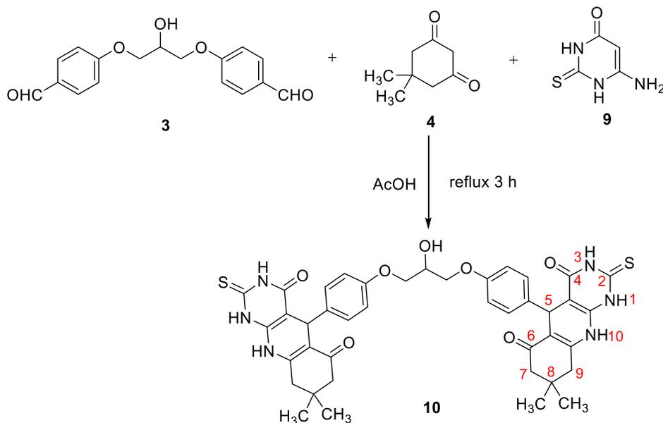
**Scheme 4.** Synthesis of bis(hexahydropyrimido[4,5-*b*]quinoline-4,6(1*H*,7*H*) dione) **10**.
