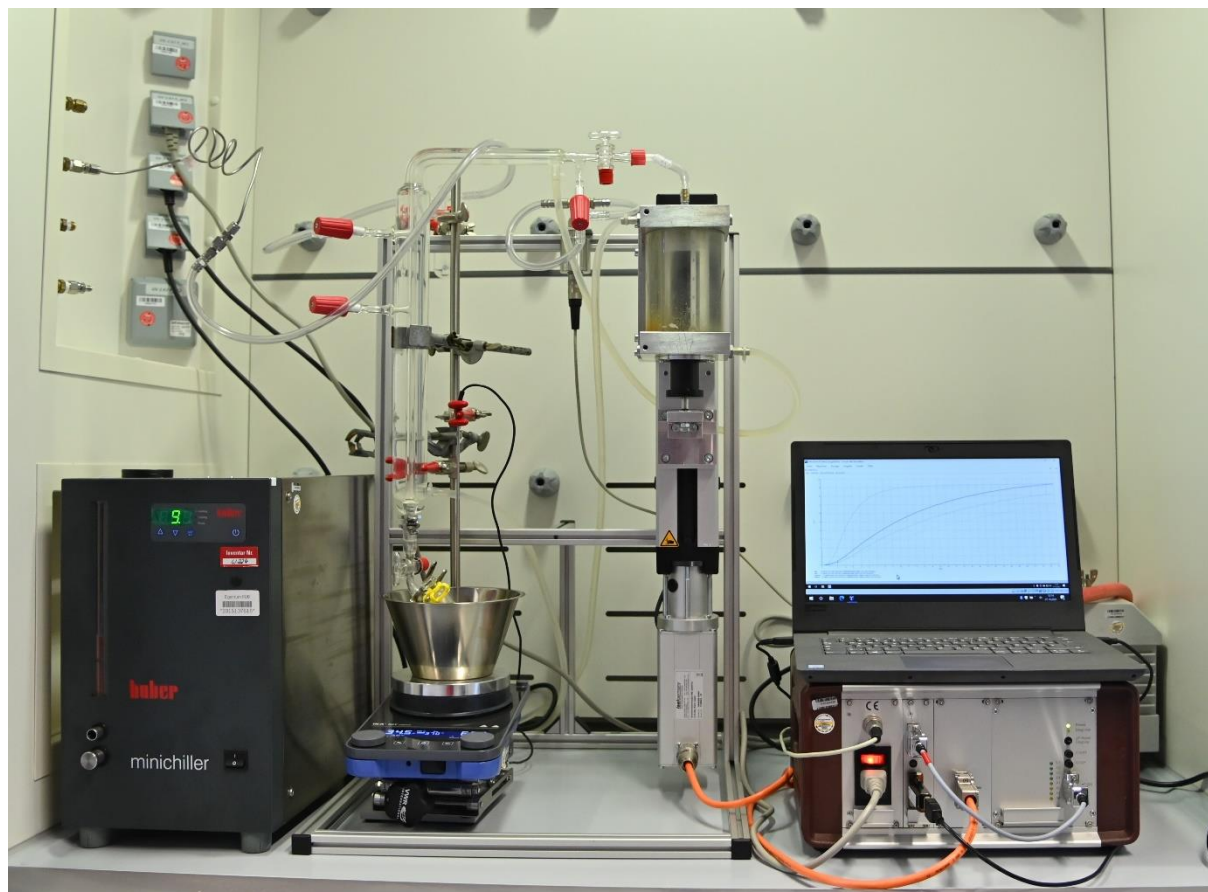
Figure S1. Volumetric gas measurement set-up (GASMESS-5) commercially available from MesSen Nord GmbH to record the evolved or consumed gas volume as a function of time.
